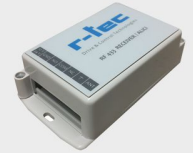
RF433 ROLLING KOD HARİCİ ALICI (230- 24 V) RF433 ROLLING CODE EXTERNAL RECEIVER (230-24 V)
