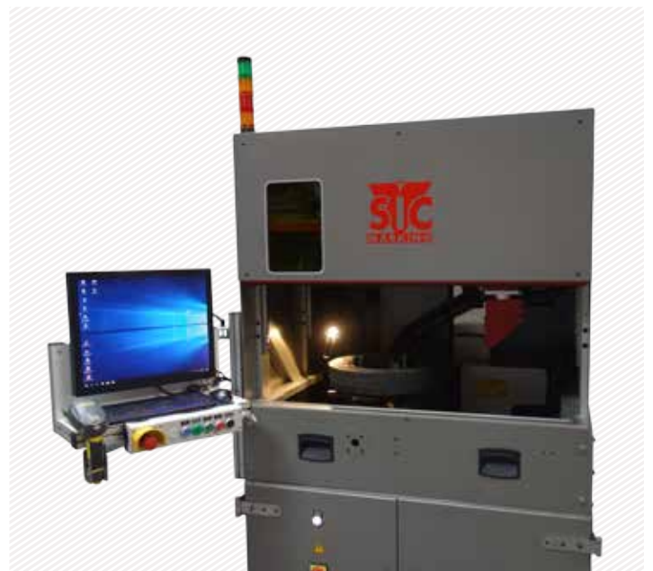
Laser station for marking three carbon brake discs inside and outside
