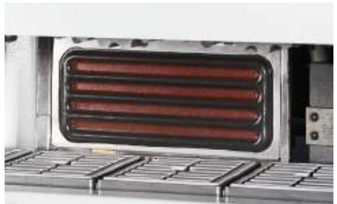
Workpiece preheating with heaters
