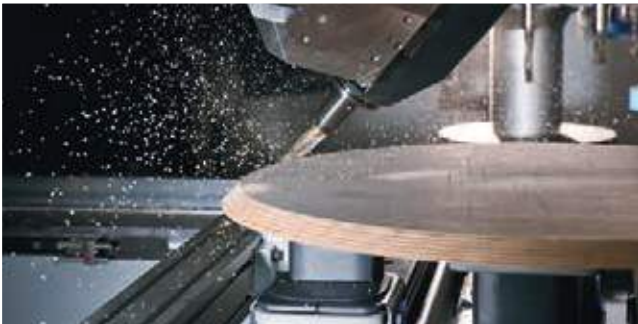
Chamfer trimming on a table top
