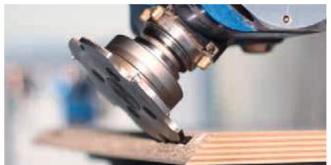
Cutting recesses for connecting fittings
