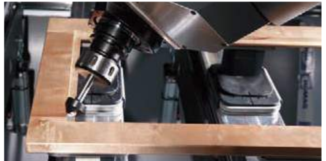
Square corner routing for a glass rebate
