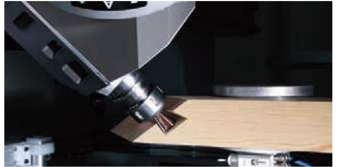
Routing of a dovetail joint for upright / transom constructions
