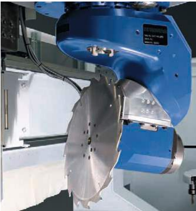
The smart DRIVE5CS 5-axis-head – compact design with short power transmission. Comprehensive technology on small space without limits regarding the processing range. Liquid-cooled spindle with 10 kW (as option 12 kW routing capacity) for efficient operations. The short design provides more space for processing (e.g. with a 350 mm saw blade, under the hood).
