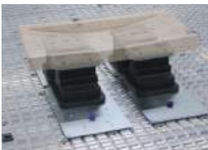
Maxi-Flex system Freely mountable system base plate for vacuum clamp.
