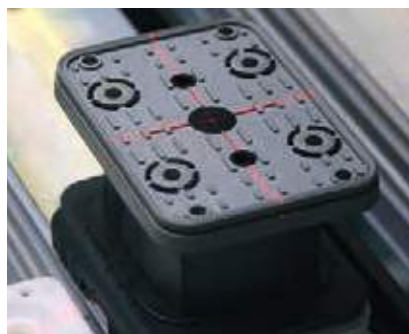
Laser positioning (optional) Simple positioning of the vacuum cups through the pin laser. The workpiece contour can be "moved" as a positioning aid for free-formed workpieces.
