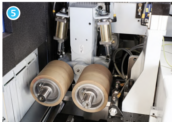
Top Pressure Rubber Rollers for sensitive surfaces after processing (Shore hardness: 80)
