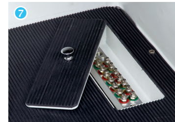
Accessible Central Lubrication at machine front
