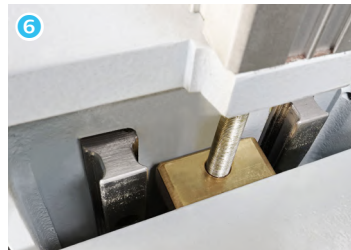
Linear Guide for precise adjustment of the top spindles and optimal work piece quality
