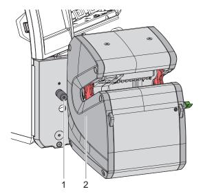
Figure 6 Pivoting the wrapper unit
