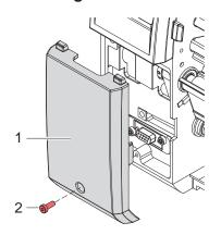
Figure 3 Removing the front cover
