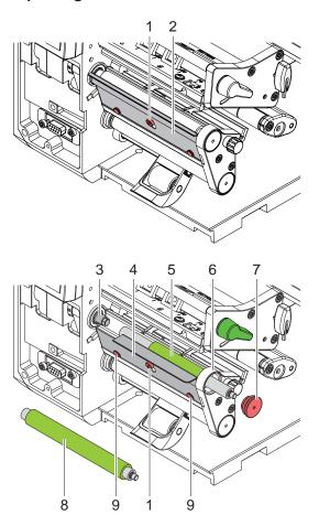
Figure 4 Replacing peel-off plate and print roller
