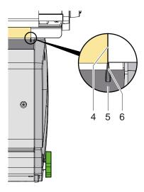
Figure 8 Setting the lateral position
