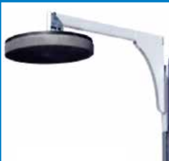
* - Option 2: Top Press (During wrapping; products that are likely to break down are fixed by pressure from the piston or motor, prevent possible damage.)
