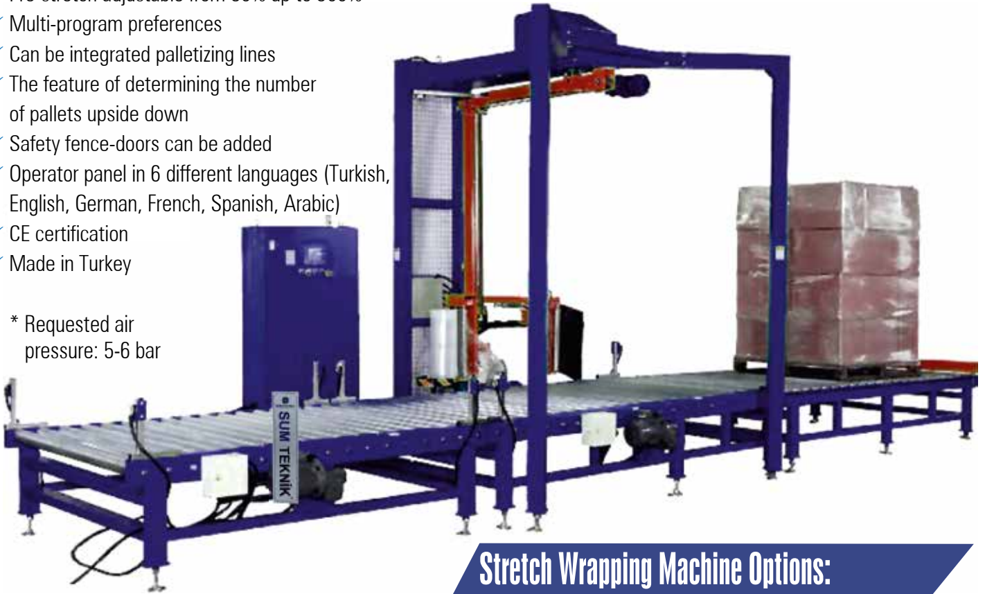
* - Option : RIP Application By turning the stretch film into a rope, it prevents the risk of overturning the products.
