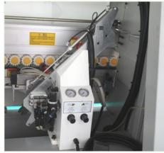
Fast move back structure, move a little backward while doing bevel edge, move forward while doing straight edge so as to achieve fast switch between bevel edge and straight edge banding work, different cutting position for two kinds of edge ensures higher edge banding quality and avoids possible collision or damage on edge tape.
