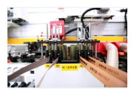
Two sets of four tapes changing system make it easy to switch between two color glue, auto changing to next position if no tape in current storage that ensures the machine continuously working without stopping.
