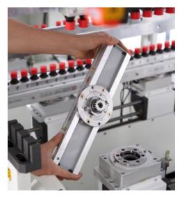
Drilling blocks with this flexibility can make different boring hole pattern easy, fast and precise.
