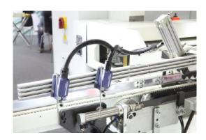
Rear positioning by servo motor and ball screw, coupled with front limit switches assures the panel stop at right position for max boring precision and positioning speed. Much faster than manual positioning provides more efficiency.
