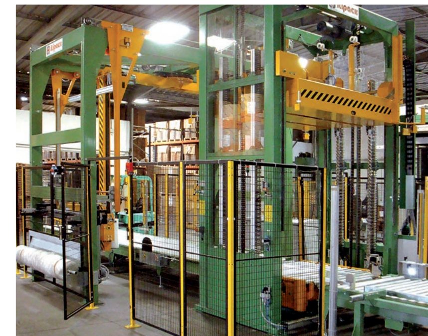
Automatic packaging line for paper sacks or cardboard with and without pallet. The displayed project is equipped with roller conveyors system, centring device station, double head top compression strapping machine, turning table to make cross strapping, automatic stretch wrapping machine and unloading conveyor sections. Each line is equipped with safety fences and light barriers
