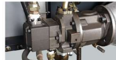
Dual Oil-circuit, Dual Oil Pump independent pump cooling oil-circuit
