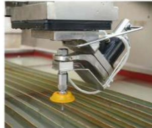
8th-gen AC 5-Axis cutting head. C-Axis rotation angle:unlimited.
