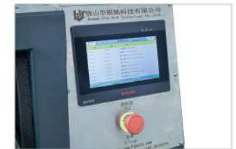
Integrated Touchscreen Monitor auto alarming system for maintenance
