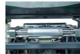
600MPa Ultra HP Intensifier working pressure could reach 460 MPa
