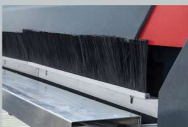
Baffle & Brush Fence stop dust entering X-beam
