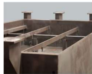
Annealing&Grit Blast Treatment makes a better fundation for cutting process
