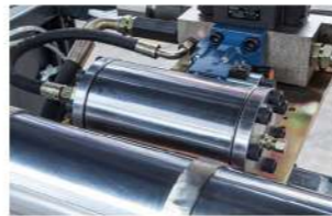
Oil-pressure Accumulator stablizing oil pressure
