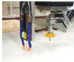
Laser altimeter assures high-accuracy bevel cutting.
