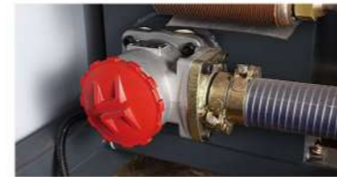
Outer Oil-filter Design much easier maintenance
