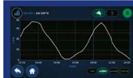
Data is stored in the internal memory and can be displayed in graphical view for each circuit. Data can also be exported for external use.
