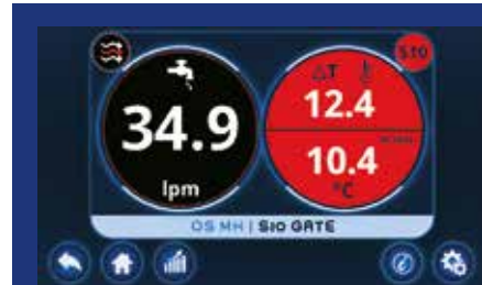
By clicking on a specific circuit you will see detailed information, including delta T (heat transfer) of the specific channel. Also, turbulent flow indicator is included.
