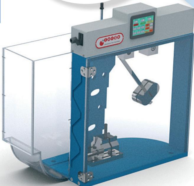
The impact test determines the breaking energy of plastics under dynamic load. There are two different test methods. Izod and Charpy test methods. The Izod impact test specimen is placed vertically while the Charpy test specimen is placed horizontally.
