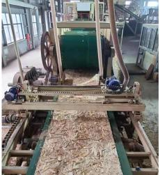
After a series of processes such as Pre-press, lengthwise saw, cross saw, accelerate conveyor, storing conveyor and loading conveyor, the rough boards are sent to loader.
