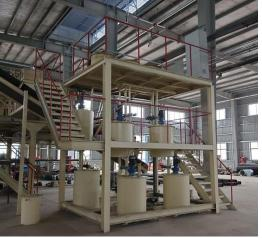
After scaled, the core and surface flakes are to be effectively and uniformly mixed with qualified glue to achieve the uniform mixing and the sufficient gluing effect.
