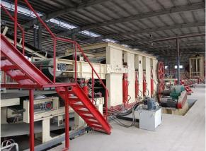
The after glued shavings are transported to the mechanical grading forming machines by the belt conveyor.and they are paved to the uniform flat slab.
