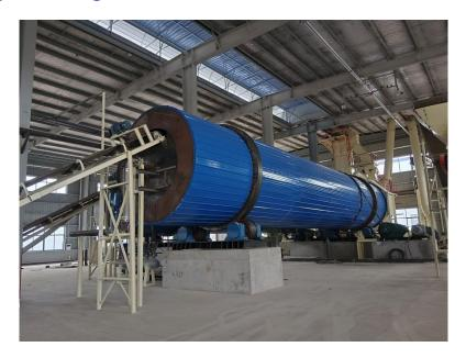
The flakes are discharged from the wet flake bin which are conveyed to the hot air dryer. Qualified core flakes are stored in core flake bin; oversize flakes are send to mill to be re-crushing, and transported to surface dry wood shavings bin to be stored.
