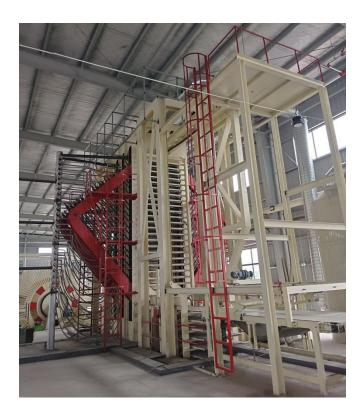
The forming boards are conveyed to the panel turnover machine to become cool, then the boards are transported to the vertical and horizontal edge cutting machine by the roller conveyor.
