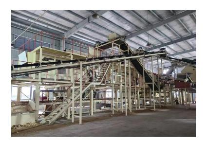
Raw material is treated by the chips making machine, then the qualified chips will be transported to the chip bin, and then feed to the ring flaker by which the chips are turned to flakes, then the flake stored in wet flake bin.
