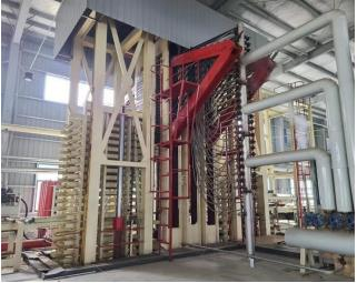
Then the mat boards are pressed by the hot press machine with suitable pressure.
