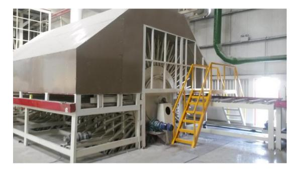
Raw board in the unloading machine will be sent to infeed roller conveyor by unloading conveyor, and then into star cooler for cooling. The cooled raw board in the star cooler will be sent by the outfeed roller conveyor into transversal and longitudinal edge saw for cutting and finally sent by dry board conveyor into lift table for stacking.
