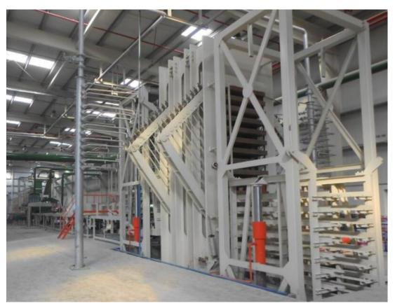
Flake applied with glue will be respectively conveyed into mechanical classi-forming machine which forms uniform and even mat. The mat will be sent to cage of loading machine through permanent magnetic separator, pre-press, edge trimming saw, cross saw, accelerating conveyor, weighing conveyor and storage conveyor and loading conveyor, etc. The cage of loading machine will send the mat into multi-opening hot press for pressing and the pressed raw board will be pushed into
