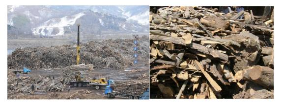
Small-diameter logs, tree branches and twigs, industrial wood residue (log cores, crushed veneer, log offcuts, plywood trimmings and waste particleboard, etc.) are used to produce gradual changing structured particleboards.
