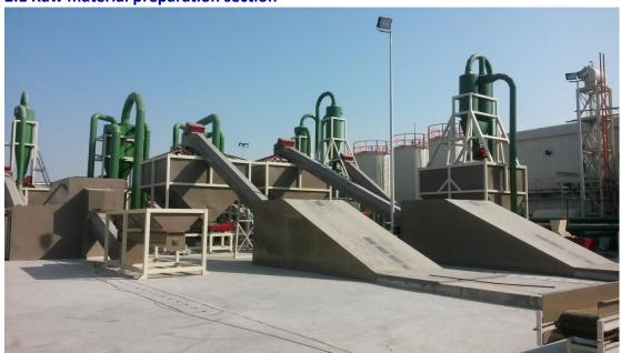
Raw material of the particle board production line after chipping and sifting treatment will be conveyed into chip silo for transit storage. Then the chip will be conveyed into flaker for flake preparation and the well prepared flake will be conveyed by conveyor into wet flake silo for transit storage.
