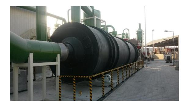
The wet flake will be conveyed by conveyor into dryer for drying and the qualified dried core-layer and surface-layer flake after sifting will be conveyed by conveyor into dry core and surface flake silo for transit storage. The oversize flake after grinding by grinder will be conveyed into dry surface flake silo for transit storage.
