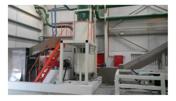
The qualified dry surface and core flake after metering respectively by flake metering silo will be conveyed into glue blender, and meanwhile, the glue blending and applying section supplies the glue which meets the requirement of the process into glue blender. With the well mixing of flake and glue by surface and core blender, it can uniformly mix and apply the glue.
