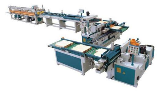
Finger Joint machine can be used for cutting teeth for the production of fine wood, furniture, etc. It is suitable for the reprocessing of waste engineering wood. It is a mechanical processing equipment to improve the utilization rate of wood and the performance of wood. It is widely used in wood processing industry, especially suitable for construction company.
