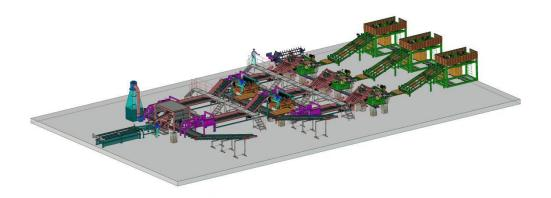
Veneer peeling production line, it processes different diameter and length logs, to make then into veneer, to supply to plywood production, blockboard production and other wood based board. Peeling machine is the main machine for plywood making. it divides into spindle and spindles type. Depend on log diameter to choose suitable veneer peeling machine.
