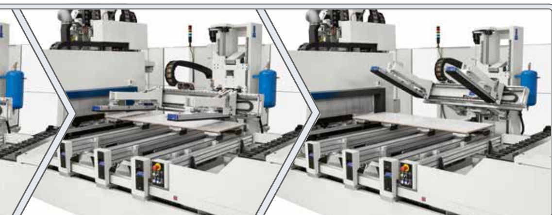
Cargo's flexible arm allows the continuous loading and unloading of workpieces in masked time, while the machine carries out the processing in the opposite area.
