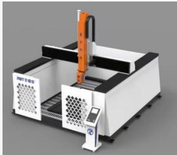
Truss-type 5 Axis CNC Machine
