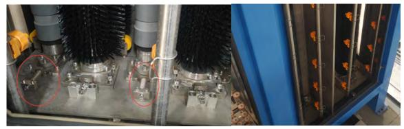
6. Drive speed adjusted by inverter stepless, the glass runs stably at proper speed.
