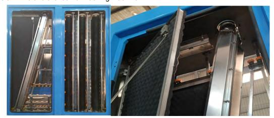
3. The washing zone and water tank are made of stainless steel and corrosion-proof material. Water heating system available.
