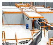
After obtaining the dimensions of the products for which surface painting is performed, the dimensions related to the unit capacity and the area to be installed, painting and drying ovens are projected in the form of a funnel or U-type in accordance with the location. High, width, height all dimensions vary. It serves both purposes.
