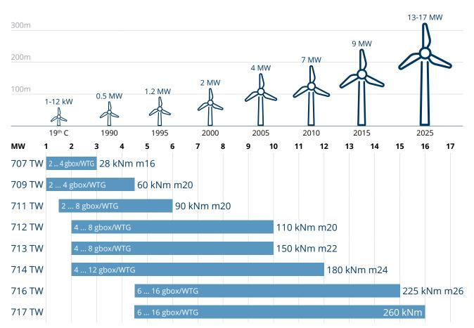
Typical application range, based on most common WTG architecture, special considerations may apply Contact Bonfiglioli for design / selection / dimensioning of pitch system
