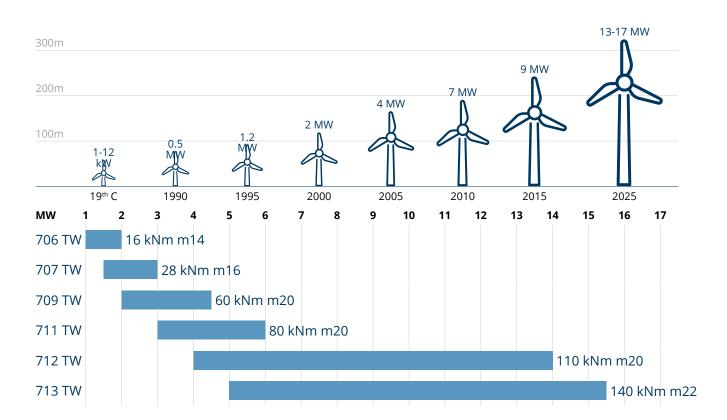
Typical application range, based on most common WTG architecture, special considerations may apply Contact Bonfiglioli for design / selection / dimensioning of pitch system
