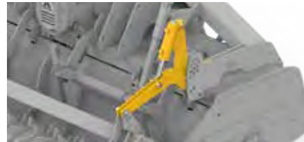
HYDRAULIC DEPTH ADJUSTMENT
