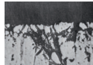
Bending test of a standard hard chrome coating. Poor adhesion, large parts of the coating have come loose.
