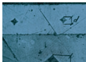
Bending test of a ductile hard chrome coating. Adhesion to the basic material is excellent, there are no cracks.
