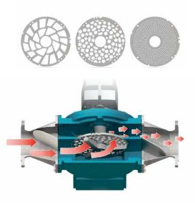
The Börger Multichopper is a perforated disk macerator with a central, perforated plate and high-performance blades for size reduction of solids contained in liquids. The macerator is available in three sizes with capacities of up to 400 m<sup>3</sup>/h.
