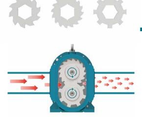
The dual-shaft grinder Multicrusher effectively and reliably processes solids contained in liquids and ensures that downstream machines and pumps operate smoothly.
