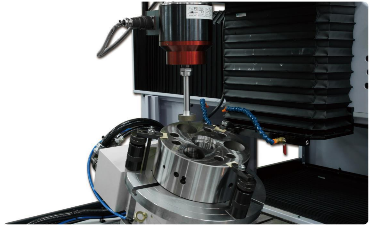
可並用第四軸作等分連續圓孔加工 Capable of synch the 4 th axis for machining process
