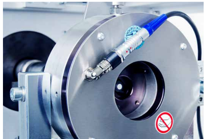
Sensor with built-in test specimen.
