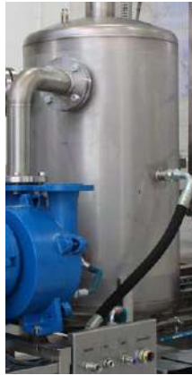
Water Scrubber Neutralization Tank
