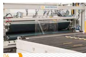
Oscillating stretch film carrier to cover all sizes with the same width of stretch film roll
