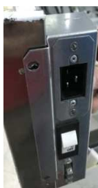
Power / on/off / dry contact
