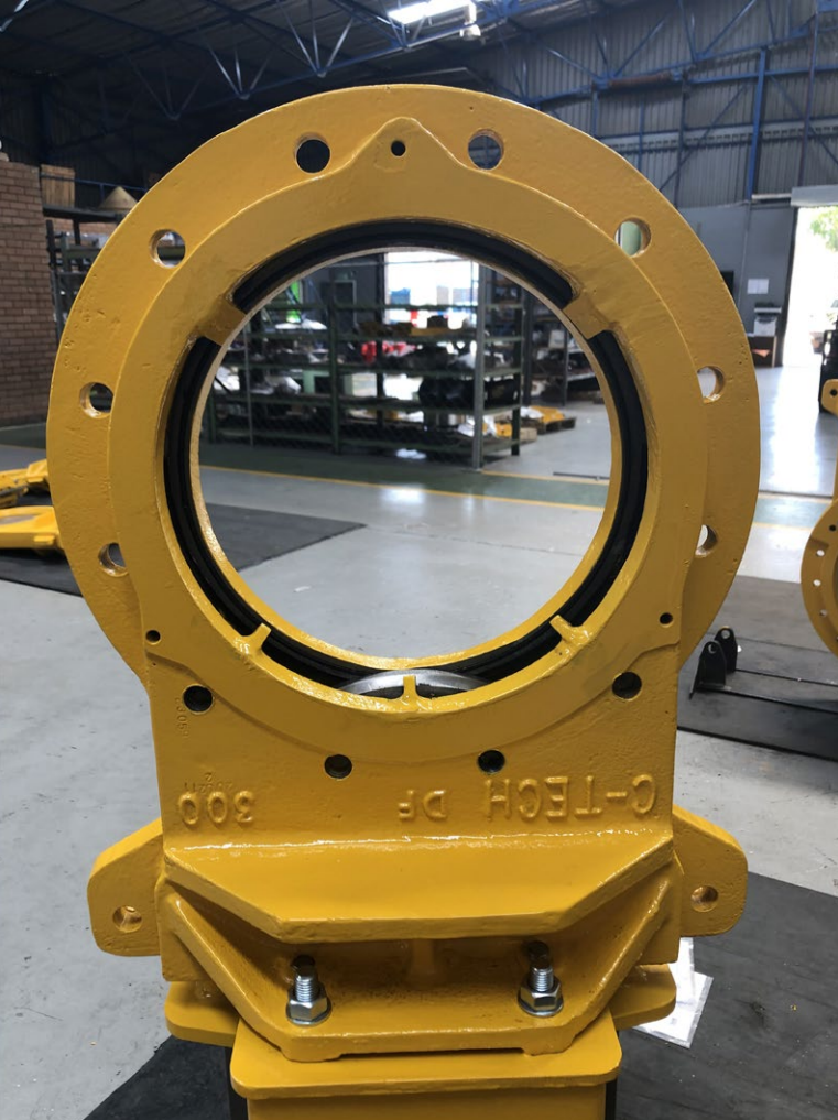
eDART Knife Gate Valve, chamfered gate fully retracted out of the flow in the open position
