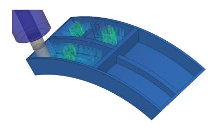
Multi-Surface Roughing of pockets with doubly-curved surfaces, offsetting from the top (ceiling) face to the bottom (floor) face using Area Clearance type machining strategies in full 5-axis.
