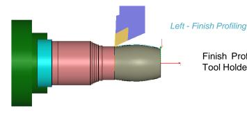
Finish Profiling also includes Undercut protection to avoid Tool Holder collision on the trailing edge whilst turning.
