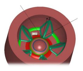
A draft function shows draft angles (tapers from the tool axis) using a similar style of graphical display as the curvature.
