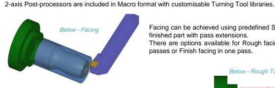
Facing can be achieved using predefined Stock or using the finished part with pass extensions.
