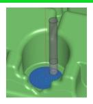
This creates an archimedean spiral toolpath from a given focal point, generating a constant contact as it machines within a given boundary. It is ideally suited for use on round shallow areas using contact angles between  $0^{\circ}-30^{\circ}$ , in conjunction with the waterline machining for the more vertical faces  $30^{\circ}-90^{\circ}$ . These passes can be constrained to a boundary or by the selected surfaces.
