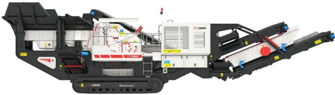
Crawler type mobile impact crusher plant
