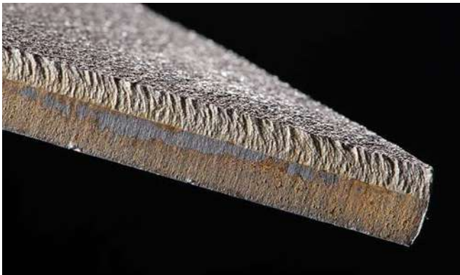
Powder coated CDP®. Visible lack of dilution.
