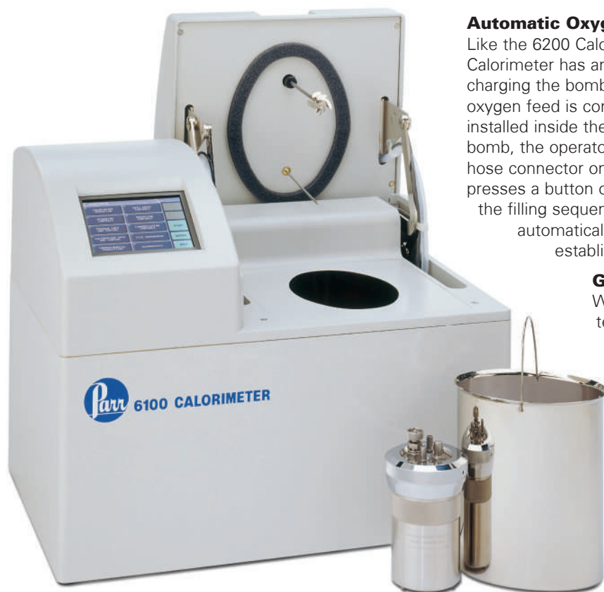
6100 Calorimeter open with 1108P Bomb and Bucket
