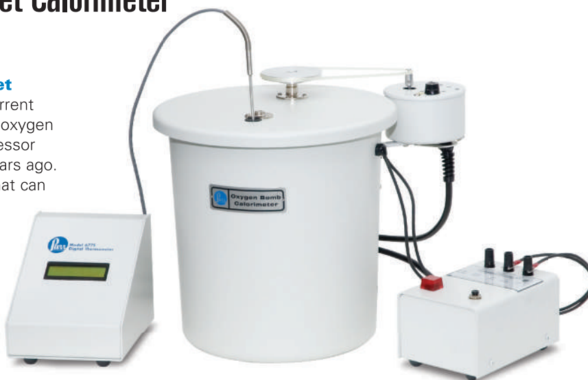
1341 Plain Jacket Calorimeter shown with 6775 Digital Thermometer and 2901 Ignition Unit.
