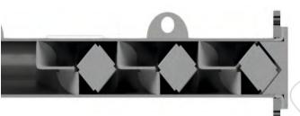
and depending on process requirements the system can have a completely sterile coating. Removable mixer elements allow cleaning from the outside. It is very practical in processing high viscosity materials. Injectors and heating cooling jackets are also available.
