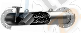
The MSM-V mixer is made of corrugated plates that form open intersecting channels through which the flow is divided into many sub-streams. The MSM-V mixer is especially used in turbulent and transitional flow regime to intensify mass transfer between immiscible fluids.
