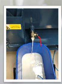
After Tap drain still much coolant left in bin. Example shows Forklift tipping bin and draining many more litres of coolant after tap drain
