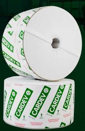
The CARDEV SDFC is a depth filter element made of long fibre cellulose, with a full diameter polyester protection disc. The element can be used on all oil-based fluids such as hydraulic, engine, gearbox oils and diesel fuels.
