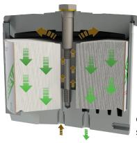
By removing up to 99.9% water contamination, the production of acids (hydrolysis) is inhibited. As the oil passes through the element, minute particles of carbon, wear metals and silicon are extracted from the oil by adhering to the many surfaces of the filter.
