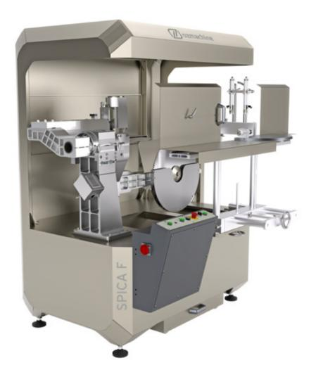
SPICA F Saw Notching Machine is designed and constructed for variable notching possibilities on the sash, frame, mullion and transom profile combinations for curtainwalls, winter gardens, skylights, and special design processing with the special angles at the profile and surface. The workpiece remains fixed on the working table and only the hydro-pneumatic sawing unit having 2 saw blades slides on the linear guides automatically to perform the notching operation.
