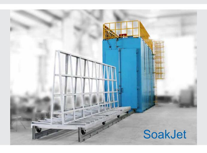
SoakJet is used by architectural glass manufacturers to test and record glass tempering quality in the post tempered glass for nickel sulfide intrusions in compliance to EN 14179-1:2005 (Glass in building. Heat-soaked thermally-toughened soda lime silicate safety glass)
