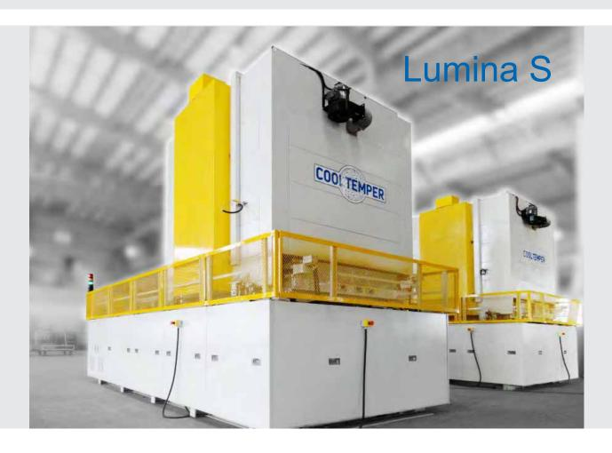
Lumina S is a low production volume chemical tempering furnace suitable for specialty products or product R&D.
