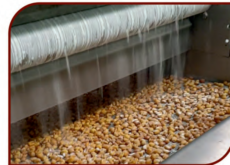
FLAVOR - SALT ADDITION SYSTEM (DOSING CONTROLLED PRODUCT SALT AND SEASONING SYSTEM)
