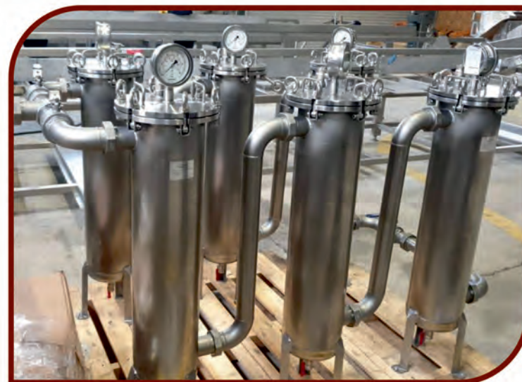
FILTER SYSTEM (FRYING OIL FILTRATION 1000 μm-250 μm)
