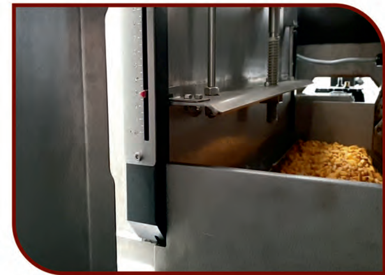
PRODUCT LAYER LEVELING ADJUSTER (FIXED LEVEL DOSING 0-100MM)
