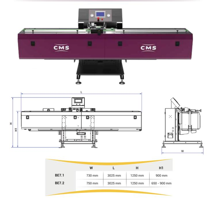
**Butyl extruder** is designed and manufactured for the application of butyl material, which provides adhesion to the edges of aluminum laths during glass joining, in the production of insulated glass.
