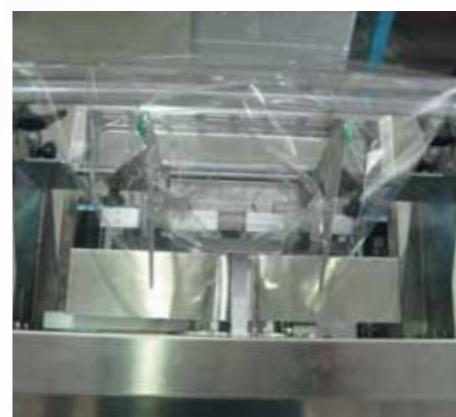
Precise product's detection thanks to barrier photocell.
