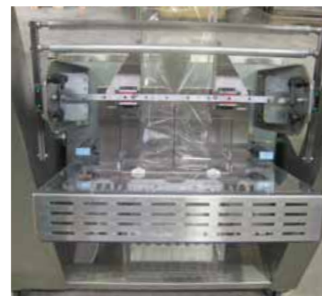
Inclinable working level from 0° to 90°.
