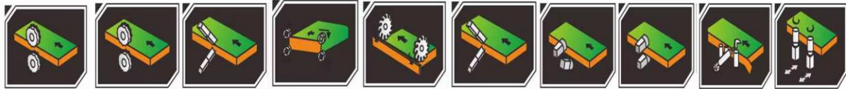
Buffing 2 Buffing 1 Flexible Scraping Corner trimming End trimming Scraping Fine trimming Rough trimming Gluing Pre-milling
