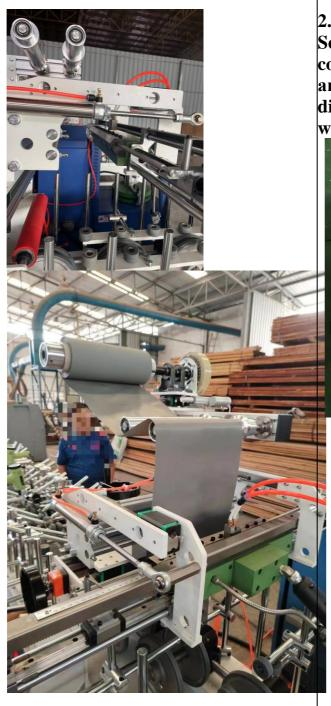
2.PUR GLUE SCRAP BLADE(350 glue width) Sealing glue cutter ,spread glue on the film ,can control the width of spread glue better, can wrap any profile , it's easy adjust width , just need to divide from middle to both sides, after finish working need to close and sealing by scotch tape .
