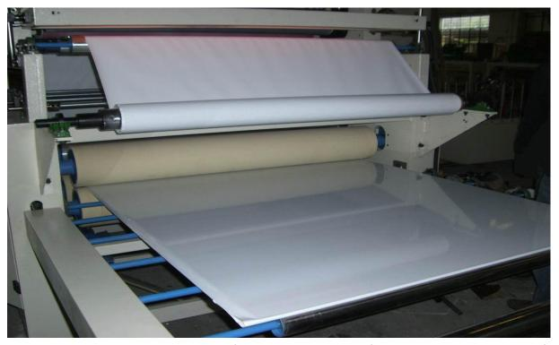
This machine is specially designed for sticking all kinds of decorative paper and pvc film on plain MDF board,chipboard and plywood.
