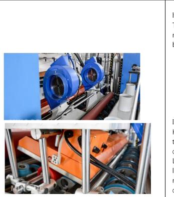
Hair dryer. Two 370W blowers are included to remove dust from corners that cannot be cleaned by the roller brushes.
