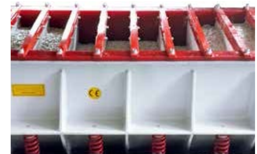
Multi separating walls application.
