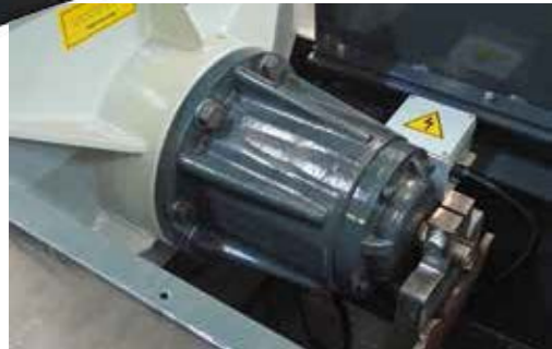
2x vibro motors are used in long machines.
