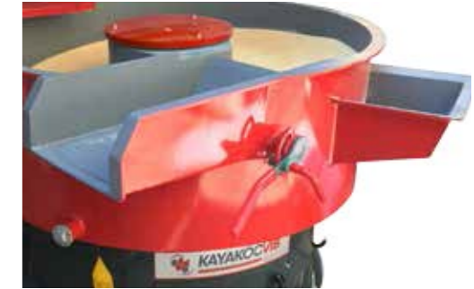
DVM, painted with epoxy paint.
