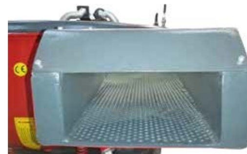
Inside of the unloading unit.
